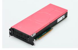
The Graphcore® C600 IPU-Processor PCIe Card is a high-performance accelerator card targeted for machine learning inference applications. Powered by the Graphcore Mk2 IPU with FP8 support, the C600 is a dual-slot, full height PCI Express Gen4 card designed for mounting in industry standard server chassis to accelerate machine intelligence workloads.
